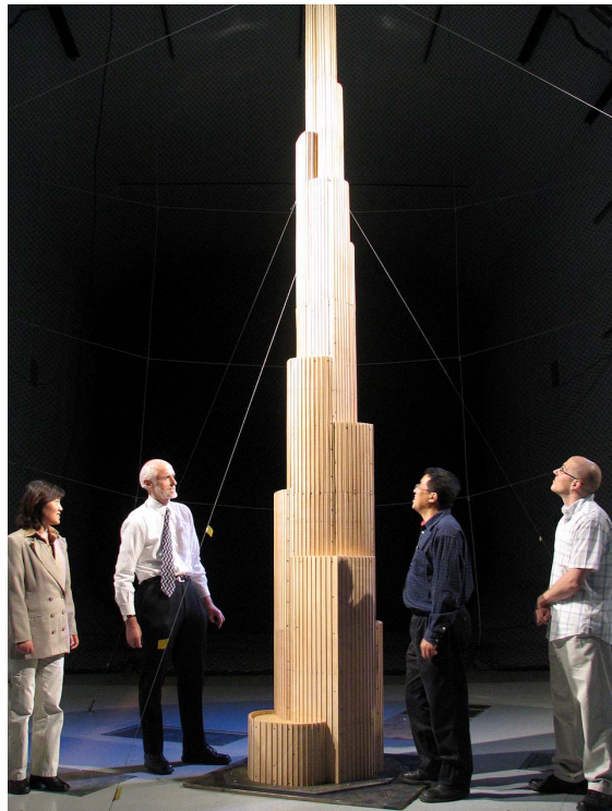
b) Rigid Pressure Tapped Model of Top Portion at 1:50 Scale.
