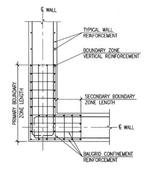
Figure 6 – Typical Boundary Zone Detail with "BauGrid" Confinement Reinforcement
