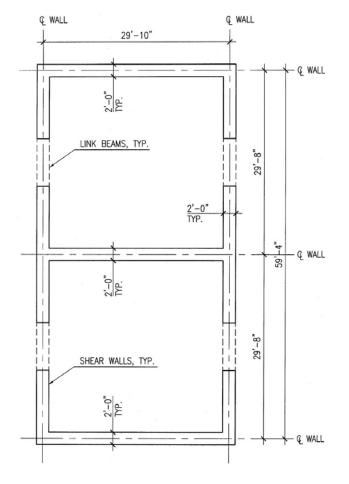
Figure 1 – Typical Shear Wall Core Plan
