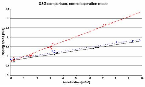
Figure 9. Tripping speed of overspeed governors as a function of the acceleration
