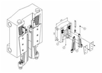
Figure 7. The KONE SGB06/07 safety gears with mechanical servo principles
