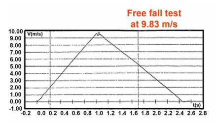
Figure 8. A typical free fall speed curve of a KONE SGB06 safety gear with mechanical servo
