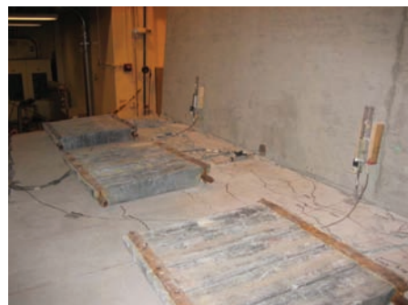
h) Cracking at Top of Slab at 5.0% Drift (Specimen Held at Peak Rotation)
