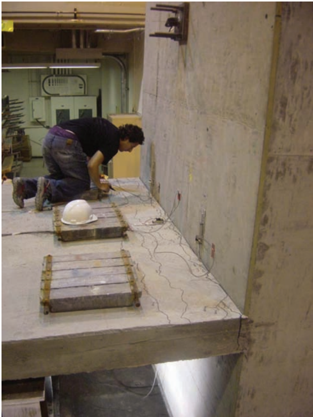
b) Cracking at Top of Slab at 1.5% Drift (Specimen Held at Peak Rotation)
