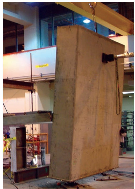
Fig. 25 – Minimum Rotation Demand in Specimens 1 &amp; 2
