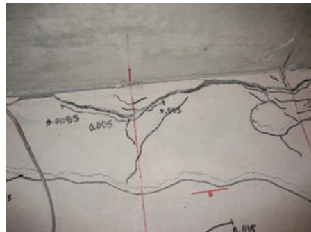
f) Cracking at Top of Slab at 2.5% Drift (Specimen Held at Peak Rotation)
