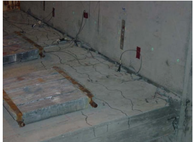
d) Cracking at Top of Slab at 5.0% Drift (Specimen Held at Peak Rotation)
