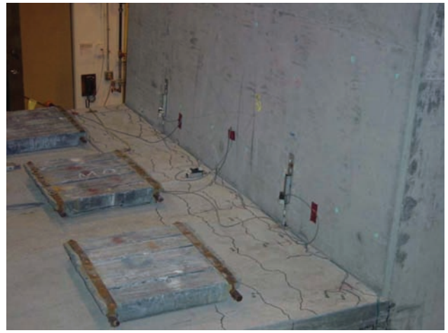
c) Cracking at Top of Slab at 2.5% Drift (Specimen Held at Peak Rotation)
