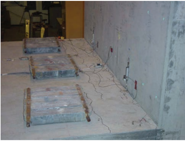
a) Cracking at Top of Slab at 0.5% Drift (Specimen Held at Peak Rotation)
