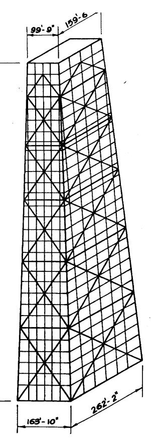
Fig. 3. Trussed-Tube Form.
