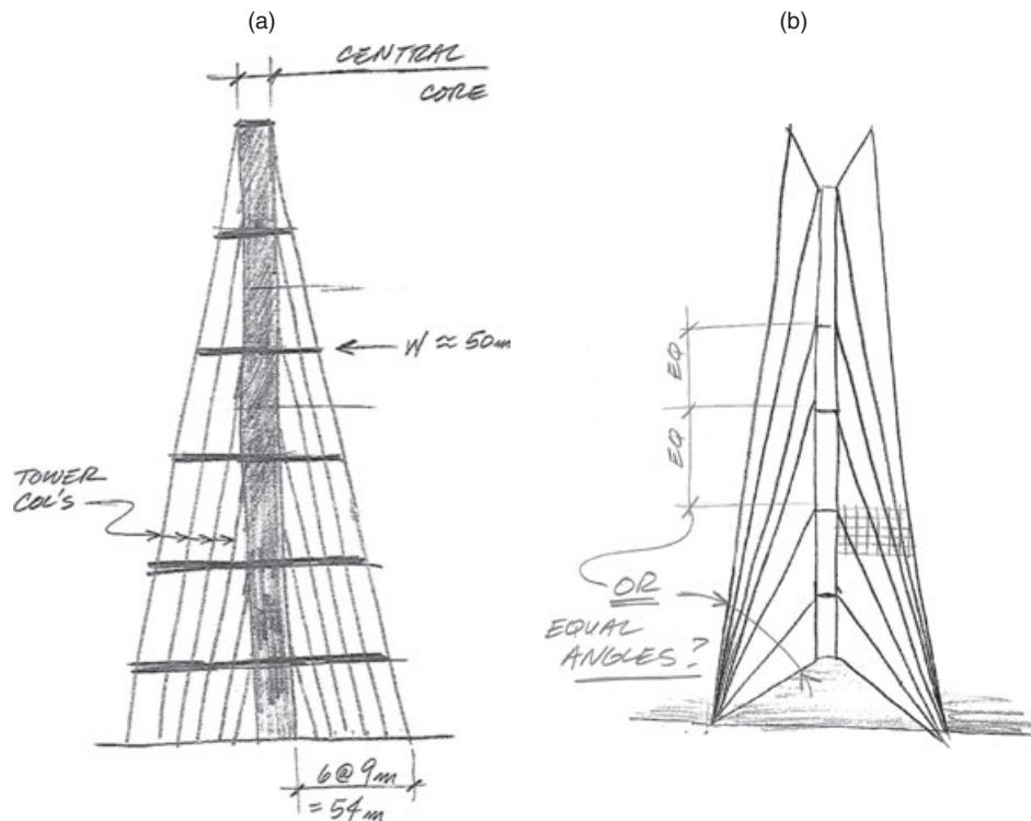
Figure 6. Reaching current structural form. (a) Parallel sloped columns. (b) Sloped columns to one point
