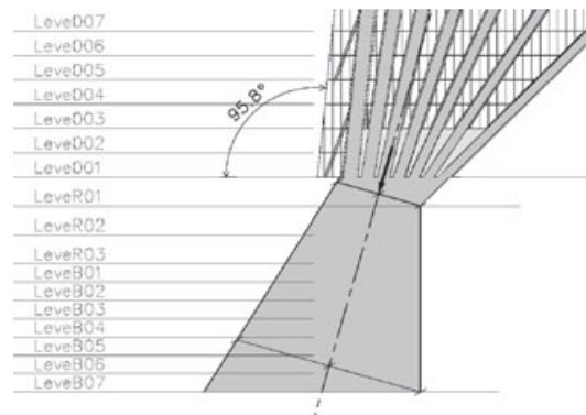
Figure 12. Fan column abutment
