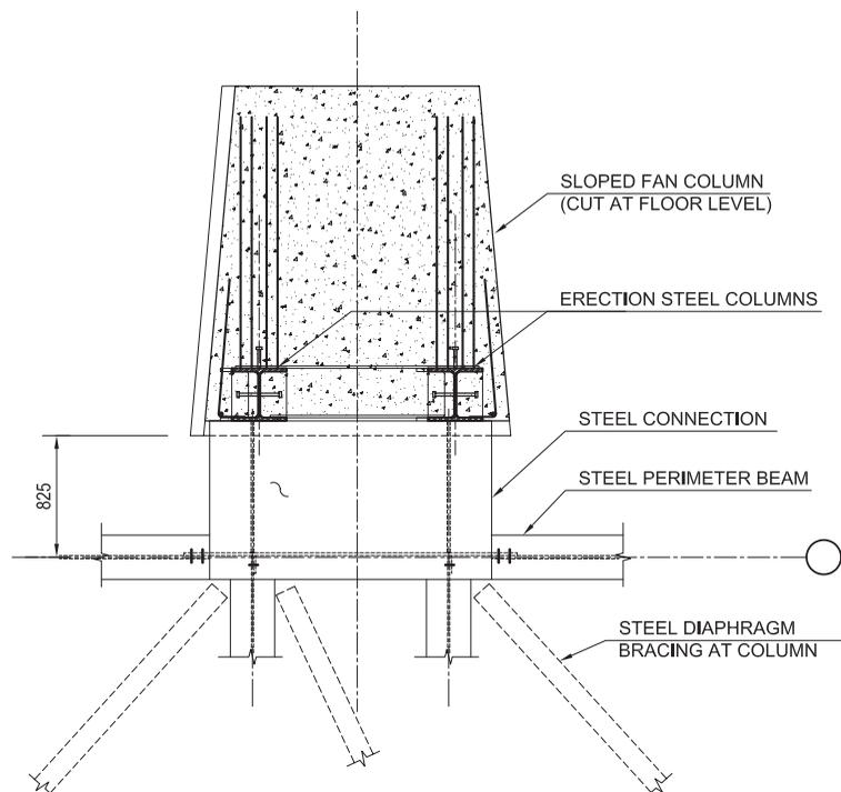
Figure 10. Connection of fan column to floor framing
