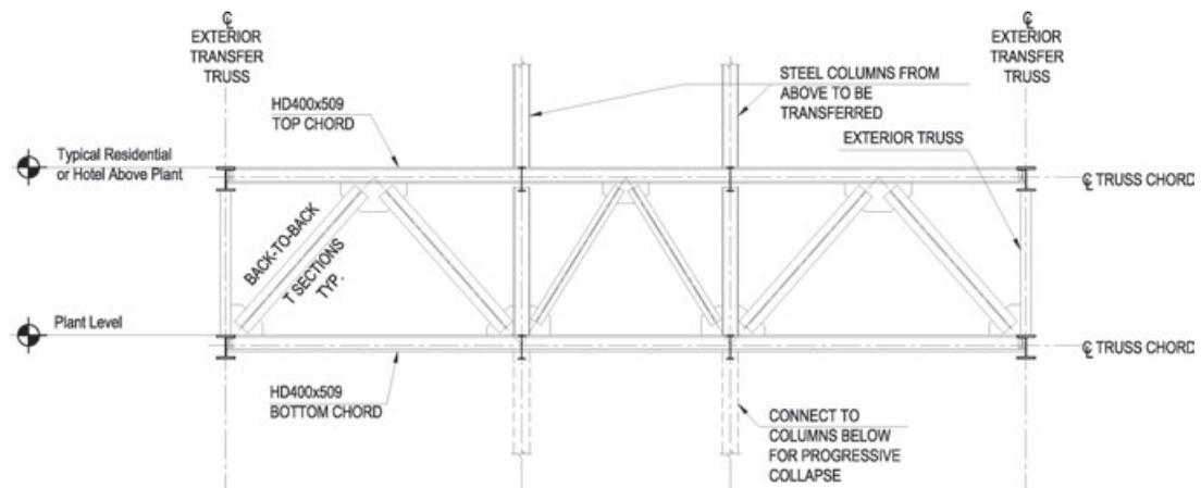
Figure 15. Full-depth transfer truss at plant levels
