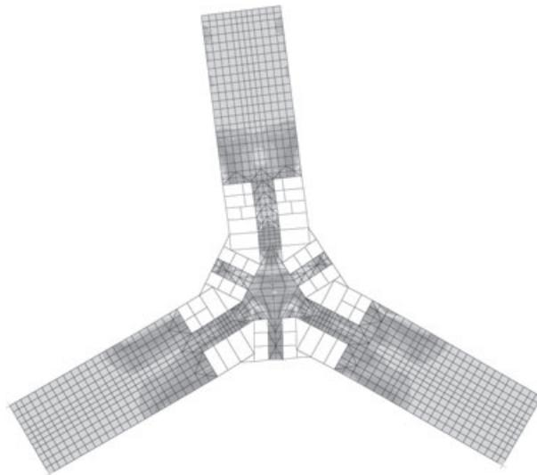
Figure 18. Diaphragm stresses due to horizontal loads
