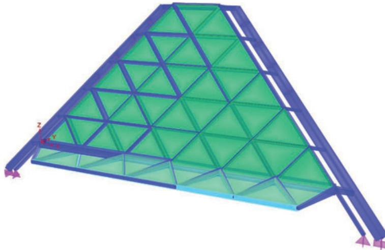
Figure 14. Structural model of atrium structural steel and glass roof enclosure
