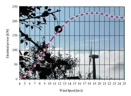
Figure 3. Electrical power versus wind speed
