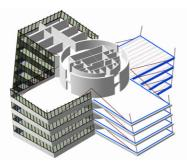
3d. Isometric drawing of cylindrical core
