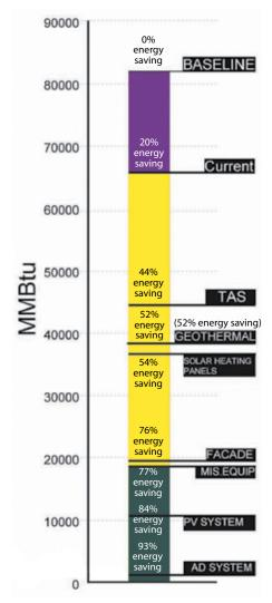
Figure 8. Overall energy footprint after all energyefficiency options are combined.
