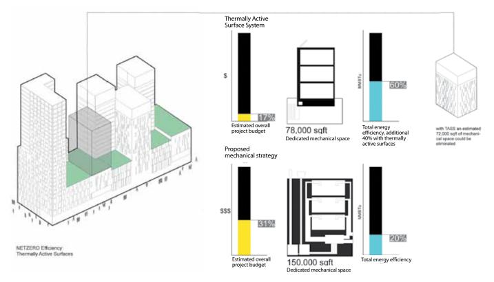
Figure 3. Heating and cooling systems comparison between forced air and Thermally Active Surface System (TASS).
