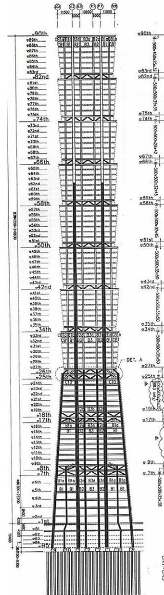
**Fig. 10.** Elevation of a perimeter moment frame line with belt trusses. Shading indicates extent of concrete fill in supercolumns.
