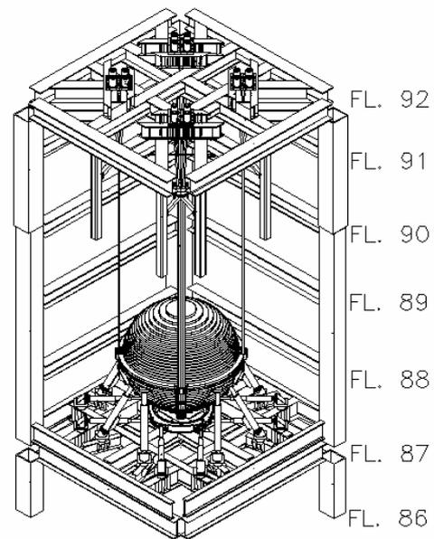
**Fig. 9.** The pendulum of the main Tuned Mass Damper, a sphere made of stacked steel plates, swings within the top floors of the highest typical building module.
