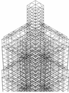
**Fig. 11.** The 3-D computer model for Taipei 101 shows core bracing, perimeter moment frames and vertical and horizontal trussing at module setbacks every 8th floor.
