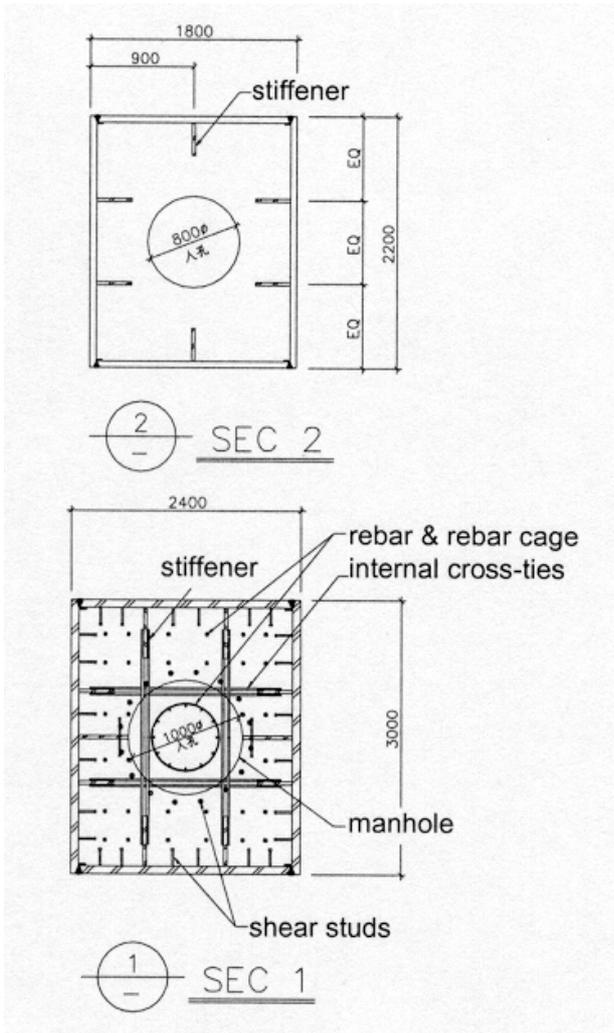
**Fig. 7.** Supercolumn box plan details show stiffeners, diaphragms, shear studs and cross-box ties.
