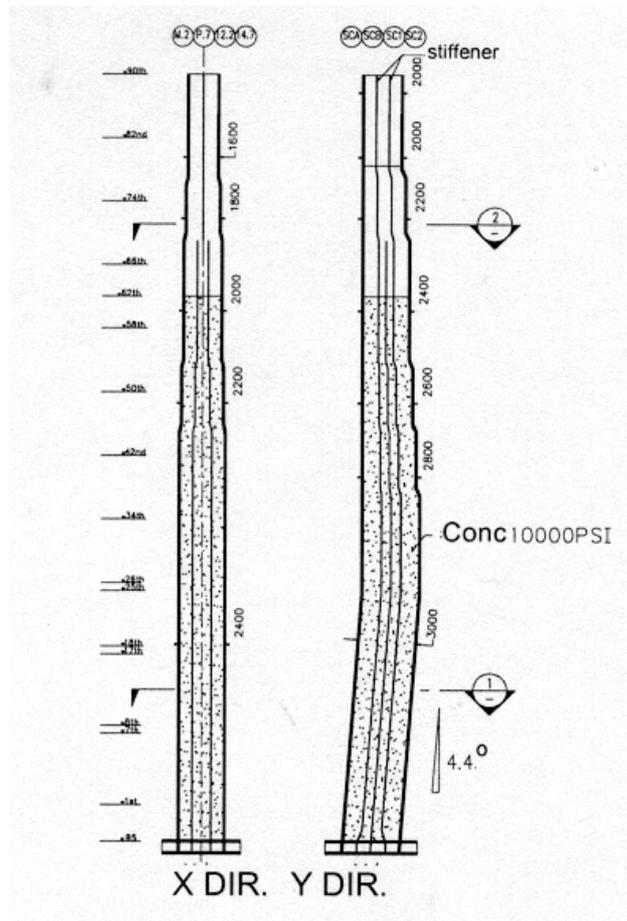
Fig. 5. Supercolumns are filled with high-strength concrete for added stiffness as shown shaded here.
