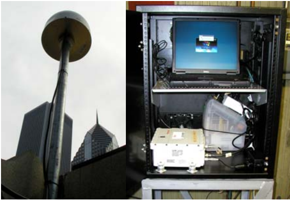
Fig.2. GPS Antenna and Supporting Electronics at Reference.
