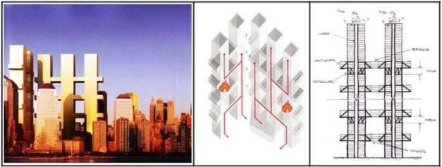
Figure 1: *Design Proposal, Richard Meier Team.* From left, (a) View across the Hudson River, (b) Evacuation diagram, (c) Structural Diagram (Source: Nordenson and Riley, 2003)
