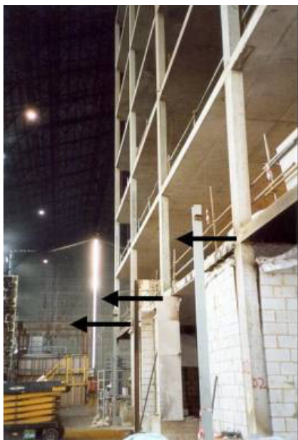
Figure 10 Lateral movement of external columns following a fire test.
