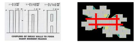
Figure 1: Giant Moment Frame used increase building's stiffness
