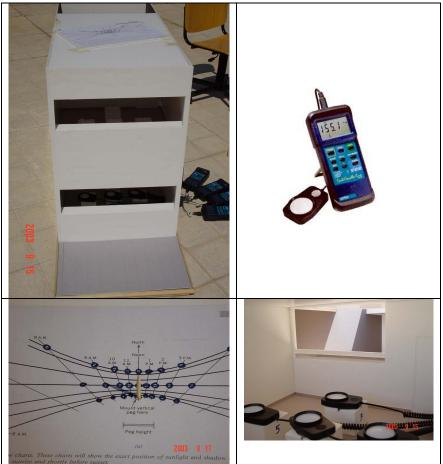
Figure 4: Simulation experiment tools used; physical model of the classrooms, Extech Instruments heavyduty light meter, peg chart used for solar angles and the photo sensors placed inside the model.
