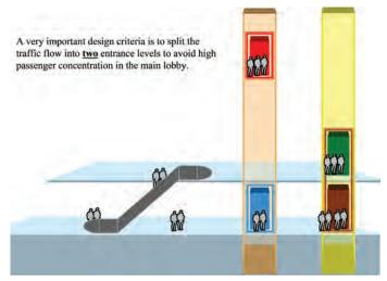
Figure 4. Concepts with TWIN and Double-Decker 图-4. 双子电梯和双轿厢电梯的概念
