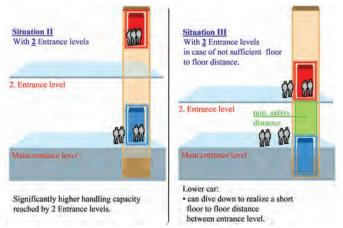
Figure 3. Flexibility of the TWIN-System with 2 cars in one shaft on floor distances 图-3. 双子电梯系统-同一井道内两个轿厢停层的灵活性
