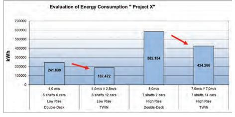
Figure 1. Evaluation of Energy Consumption 图-1. 能量消耗评估
