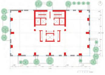
Figure 3. Horizontal section of the typical floor plan of the Tower E The structure of the Bosco Verticale is made entirely of reinforced concrete. The vertical load-bearing structures are formed by 13 pillars, placed on the perimeter of the floor plan, and by the service core, containing two staircases, three lifts and five ducts for the systems. 图3. 塔E标准层平面图
