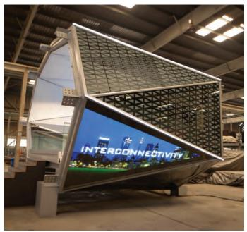
Figure 8. Prototype of a typical module with high resolution external screen solution 图8. 安装了高分辨率外屏幕的典型模块
