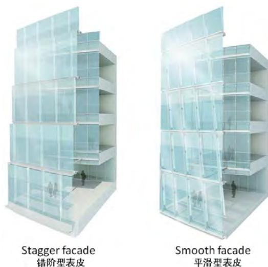
Figure 2.14. The difference between a staggered versus a smooth façade design. (Source: Gensler) 图2.14. 上海中心大厦平滑幕墙与交错式幕墙设计 (来源: Gensler)
