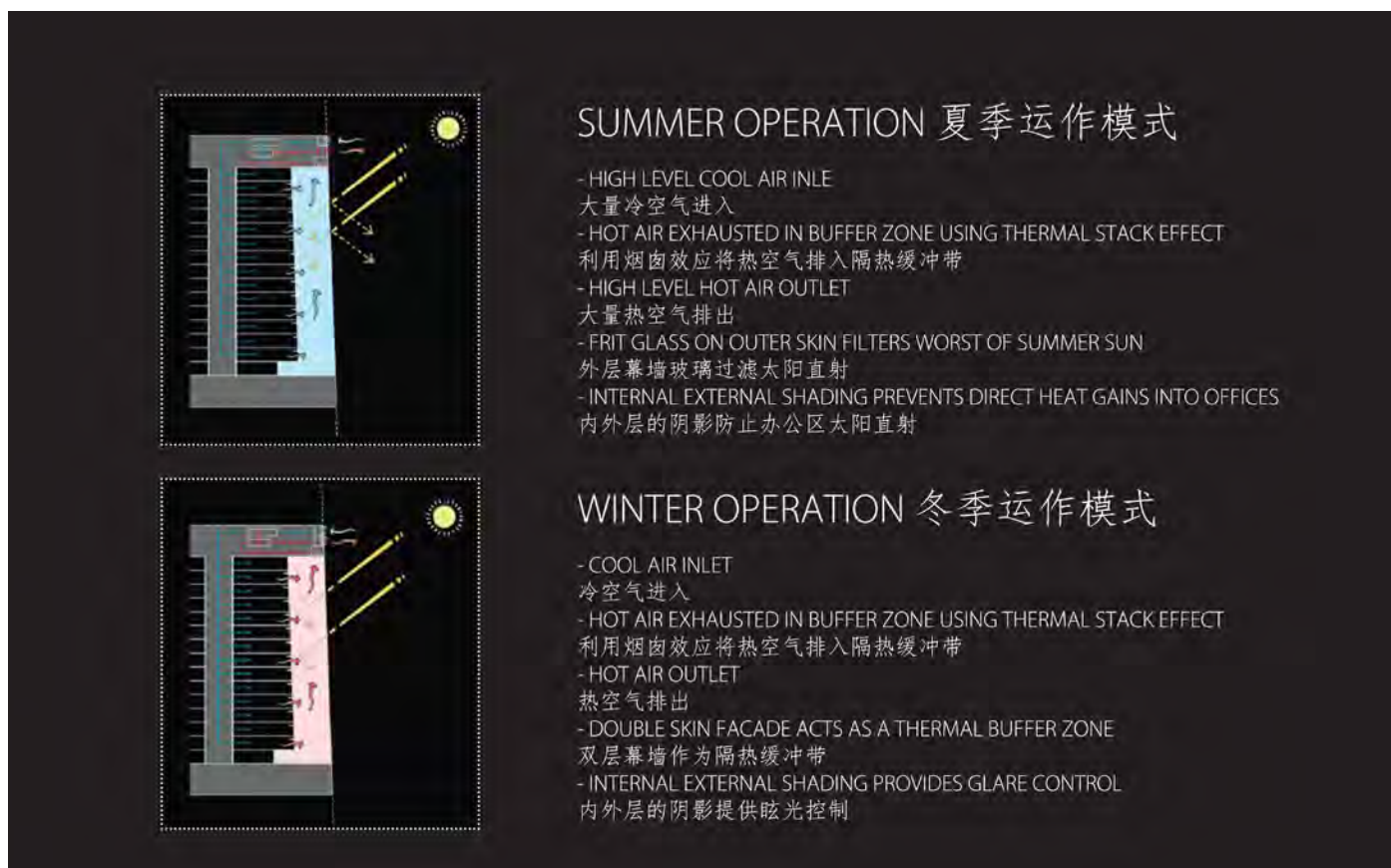
Figure 3.36. Modes of operation for the double façade at Shanghai Tower. (Source: Cosentini)
