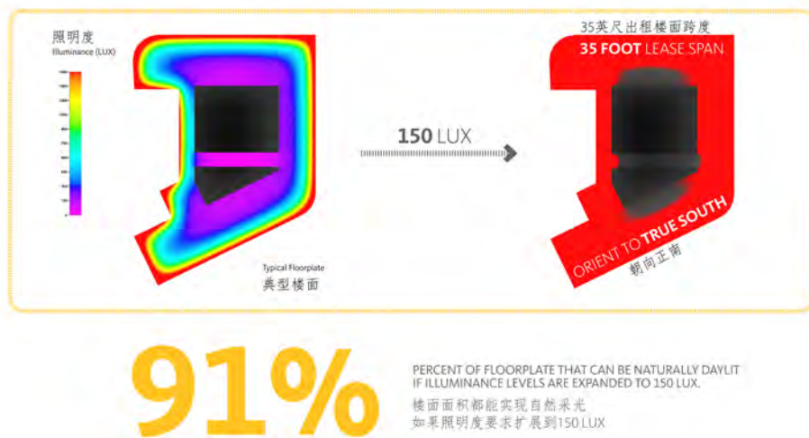
Figure 3.29. Daylight evaluation for The Tower at PNC Plaza (Source: Gensler) 图3.29. PNC广场塔楼自然采光评估 (来源: Gensler)
