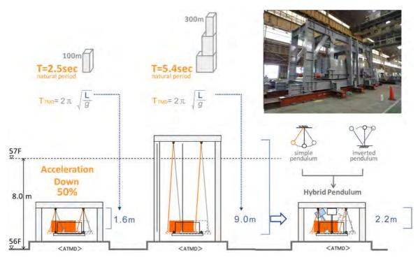
Figure 33. Illustration overview of hybrid pendulum ATMD.
