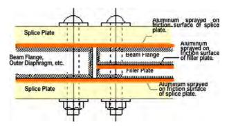
Figure 21. Aluminum spray jointing.
