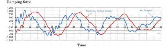
Figure 26. Two types of dampers working with lag between their most effective time.
