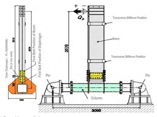
Figure 19. Test article - outer diaphragm.
