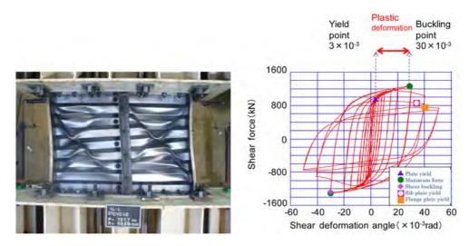
Figure 30. Photo of corrugated steel plate wall (left) and chart of load-deformation relations with excellent energy absorptions (right).
