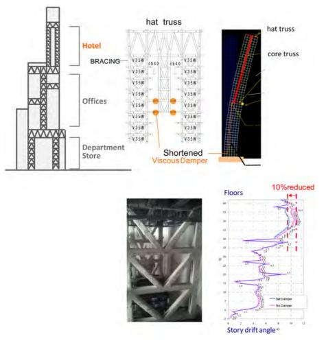
Figure 31. Mechanism of Core Truss Damper.
