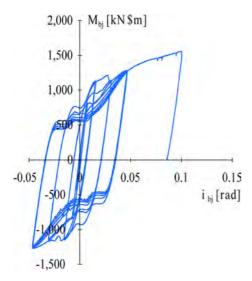
Figure 20. Load-deformation relations.
