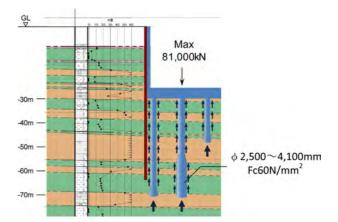
Figure 13. Elevation of piles.
