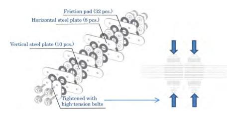
Figure 27. Mechanism of rotational friction damper.
