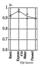
Figure 22. Relations between construction troubles and slip factors.
