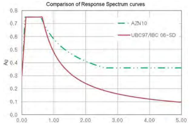
Figure 7. Comparison of Response Spectrum Curves, (AZN vs UBC/IBC).
