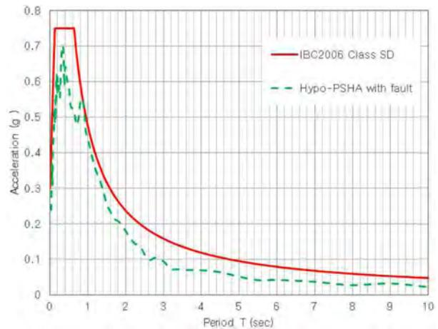
**Figure 10.** Comparison of design horizontal response spectra with fault underneath the Site.
