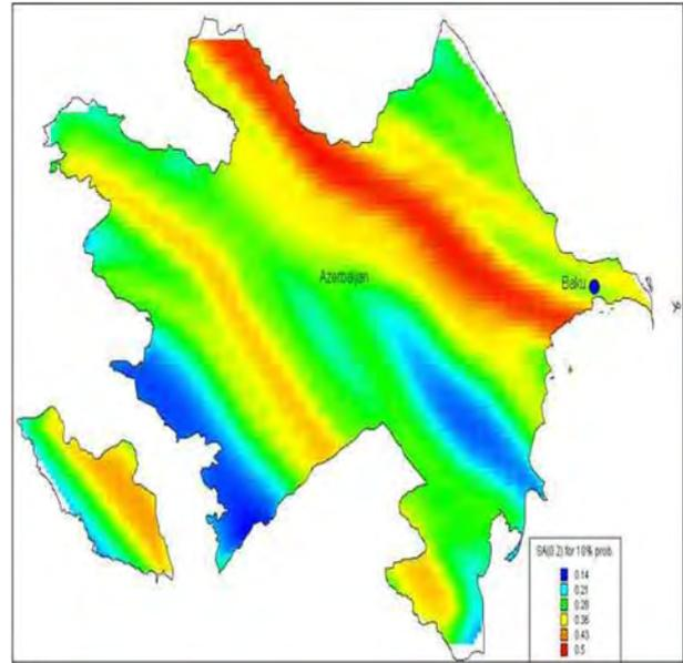
**Figure 3.** Spectral Acceleration for P = 0.2 sec with a Return period of 475 years by Akhundov et al. (2011).
