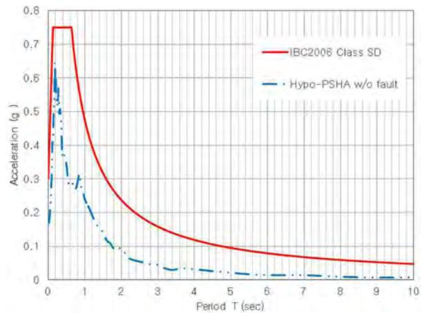
**Figure 9.** Comparison of design horizontal response spectra.
