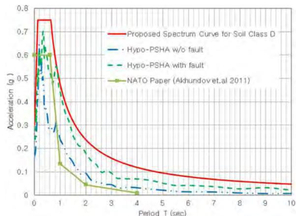
**Figure 11.** Comparison of Response Spectra.
