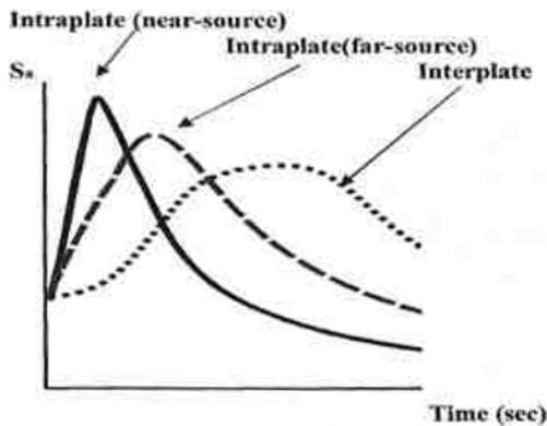
**Figure 8.** Comparison of Inter and Intra-Plate Earthquakes by Gioncu, Mazzolani (2011).
