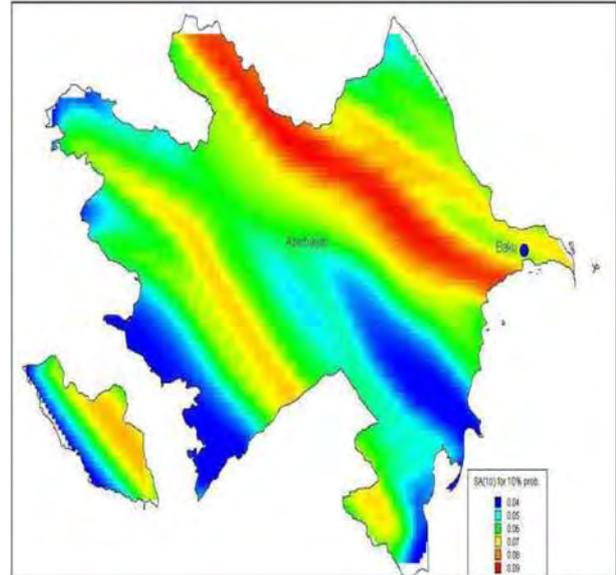
**Figure 4.** Spectral Acceleration for P = 1.0 sec with a Return period of 475 years by Akhundov et al. (2011).
