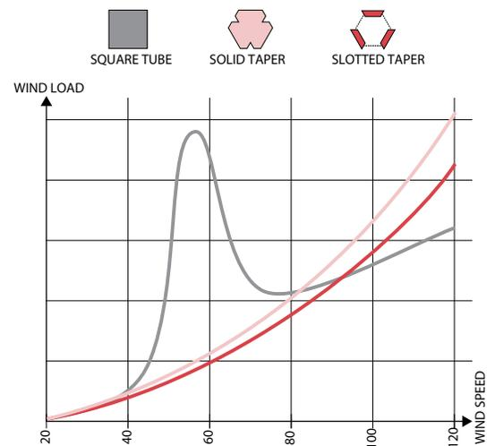
Figure 10. Wind response of three primary tower types. © RWDI
