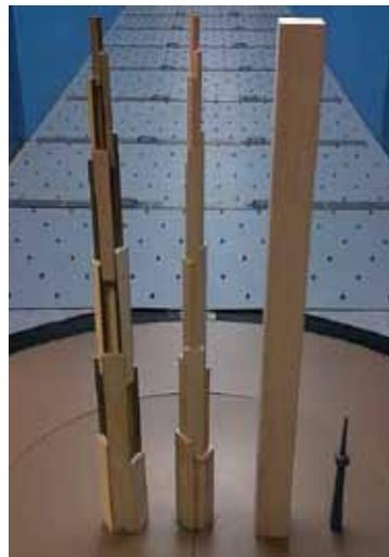
Figure 9. Wind response was tested on models for three primary tower types. © RWDI
