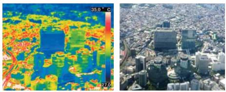
Figure 14. Aerial thermographic photo of the BioSkin-clad building. © Nikken Sekkei
