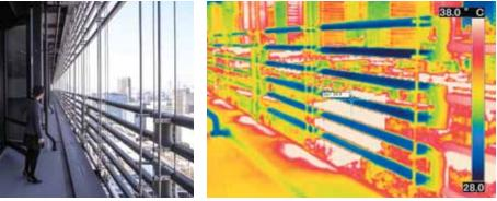
Figure 13. Thermographic photo of NBF Osaki Building's façade after the BioSkin was activated. © Gankosha
