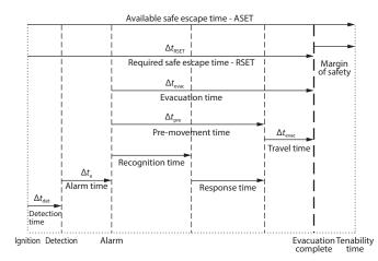
Figure 4. Example of a timeline comparison of the Available Safe Egress Time (ASET) and Required Safe Egress Time (RSET). Source: PD 7974-6:2004.
