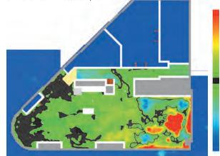
Figure 9. Temperature in Level 33 shortly after sprinkler activation. Red shows high temperatures (100°C or more), blue shows low temperature (20–35°C).
