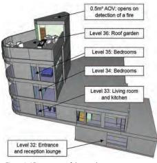
Figure 3. 3D geometry of the penthouse.
