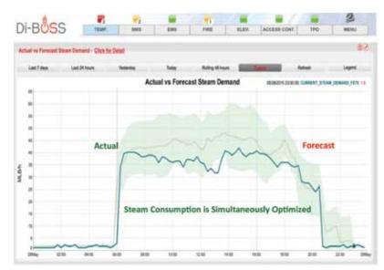
Graph 8: Di-BOSS TPO forecast (red), derived from steam consumption on previous days with similar weather, if operational realities allow. Source: Rudin Management Company. Inc.
