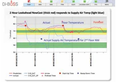
Graph 10: The Di-BOSS TPO uses a 2-hour lookahead called the "NowCast" (bold red) to forecast space temperatures for tenants based on the current supply air temperature (light blue). Source: Rudin Management Company, Inc.
