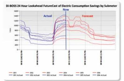
Graph 5: Electricity consumption savings that are constantly monitored on 6 submeters at 345 Park Avenue. Blue is the actual consumption and red is the 24 hour FutureCast. Source: Rudin Management Company, Inc.
