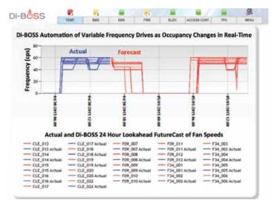
Graph 4: Actual VFD frequencies for the current day (blue) are constantly compared to the 24 hour "FutureCast" of frequencies for tomorrow (red) so that the feedback from any errors can be learned from and corrected by the TPO. Source: Rudin Management Company, Inc.
