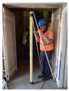
Figure 2. Height is measured from the level of the lowest, significant, open-air, pedestrian entrance to the architectural top of the structure (CTBUH criteria).
