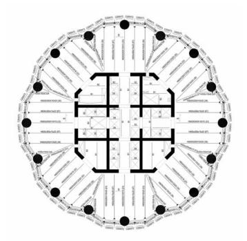
a center core with additional shear walls outside of the core, or a center core and perimeter moment frames. For a tower of this height, Chinese building codes do not permit the use of just a shear wall system. Perimeter moment frames must be used together with the core.
