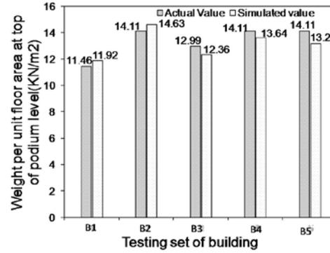
Figure 4.4 Comparison of actual weight per unit floor area of tower of test building with simulated from artificial neural network.
