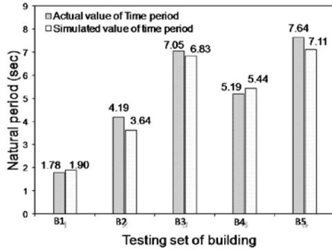
Figure 4.1 Comparison of natural period of test buildings with simulated natural periods from artificial neural network.
