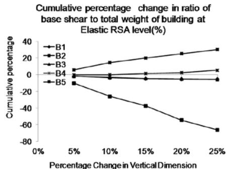
Figure 4.16 Changed in ratio of base shear to total weight of building at RSA elastic level of test building simulated by Network VIII with vertical dimension of building keeping horizontal dimension of building and dimension of shear wall constant.
