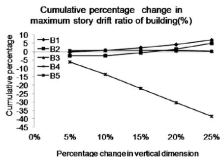
Figure 4.15 Changed in maximum story drift ratio at top of podium level of building simulated by Network VII with vertical dimension of building keeping horizontal dimension of building and dimension of shear wall constant.
