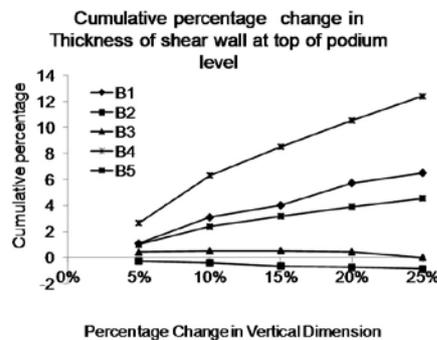
Figure 4.14 Changed in Thickness of tower at top of podium level of building simulated by Network VI with vertical dimension of building keeping horizontal dimension of building and dimension of shear wall constant.
