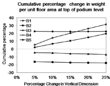
Figure 4.12 Changed in weight per unit floor area at top of podium level of building simulated by Network IV with vertical dimension of building keeping horizontal dimension of building and dimension of shear wall constant.
