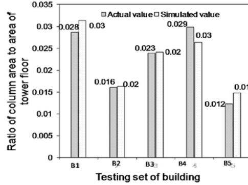
Figure 4.2 Comparison of actual ratio of total area of column to total area of tower of test building with simulated from artificial neural network.
