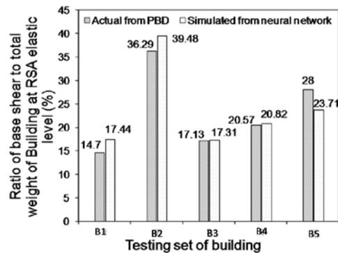
Figure 4.8 Comparison of actual ratio of base shear to total weight of building at RSA elastic level and simulated from artificial neural network.
