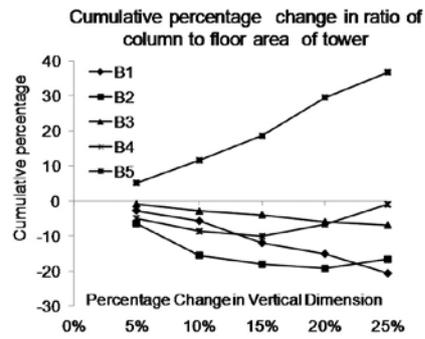
Figure 4.10 Changed in ratio of total area of column to total area of tower of test building simulated by Network II with vertical dimension of building keeping horizontal dimension of building and dimension of shear wall constant.
