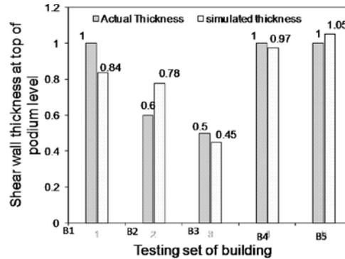
Figure 4.6 Comparison of actual shear wall thickness of test building with simulated from artificial neural network.
