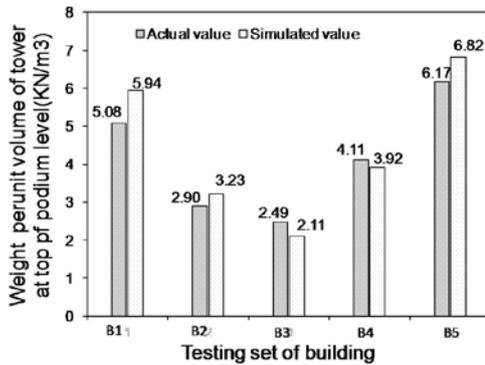
Figure 4.5 Comparison of actual weight per unit volume of tower of test building with simulated from artificial neural network.
