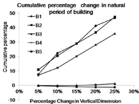
Figure 4.9 Changed in Natural period of building simulated by Network I with vertical dimension of building keeping horizontal dimension of building and dimension of shear wall constant.
