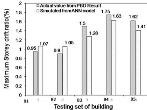
Figure 4.7 Comparison of actual Maximum storey drift ratio of test building with simulated from artificial neural network.
