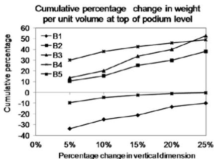
Figure 4.13 Changed in weight per unit volume of tower at top of podium level of building simulated by Network V with vertical dimension of building keeping horizontal dimension of building and dimension of shear wall constant.
