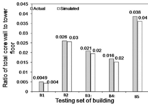
Figure 4.3 Comparison of actual ratio of total area of core wall to total area of tower of test building with simulated from artificial neural network.
