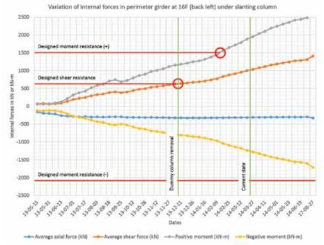
Figure 11. Variation of internal forces in the cracked perimeter girder at Level 16 (Source: Daewoo E&C)
