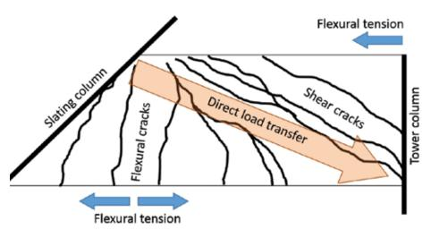
Figure 12. Assumed mechanism of direct load transfer from slating column to tower column in the short perimeter girders (Source: Daewoo E&C)
