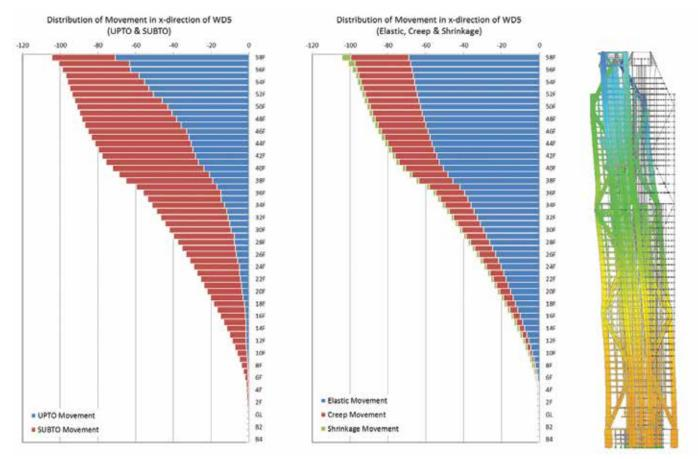
Figure 7. Results of construction stage analysis of the Tower regarding deviation from verticality (Source: Daewoo E&C)
