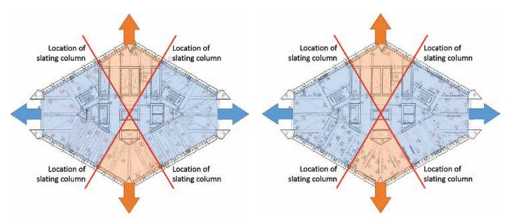
Figure 13 Crack patterns and in-plane tension caused by overall building behavior: for floor slab (above) and for girders and beams (below) (Source: Daewoo E&C)
