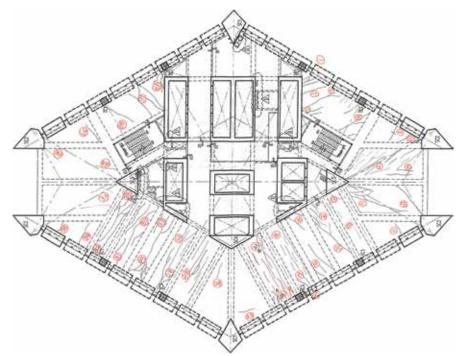
Figure 3. Map of cracks on the soffit of floor slab at Level 16 (Source: Daewoo E&C)
