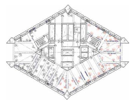
Figure 5. Map of cracks in perimeter girders and beams connecting perimeter girders and core walls at Level 16 (Source: Daewoo E&C)
