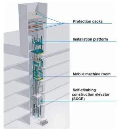
Figure 3. The SCCE provides an engineered solution that is adaptable to almost any high-rise building (Source: KONE)
