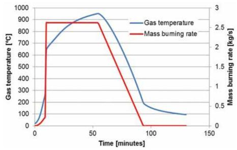
Figure 4. Main results of the worst case realistic compartment fire (Source: BuroHappold Engineering)
