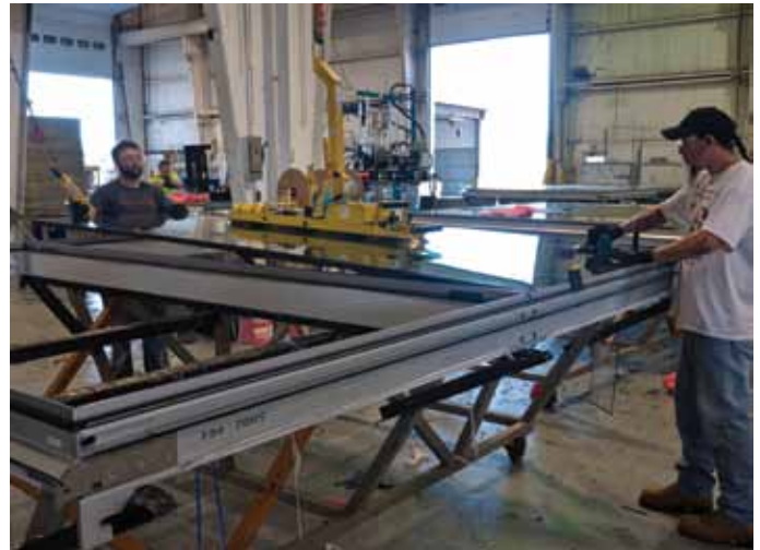
Figure 2. Curtain wall units in production at an assembly plant where quality can be better controlled than on the building site. (Enclos Corp)
