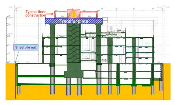
Figure 17. Typical Cross-section along N-S direction.
