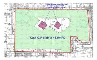
Figure 19. Local Excavation for Inner Pile Caps.
