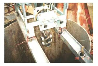
Figure 2. Koden (Sonar) Testing.
