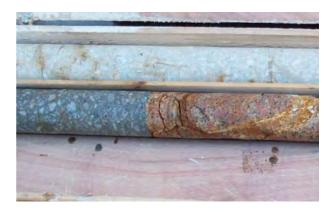
Figure 4. Concrete/bedrock interface.
