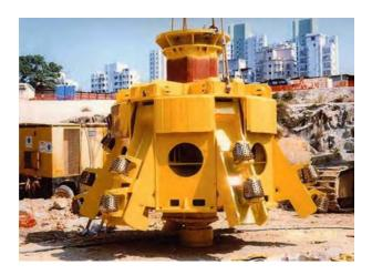
Figure 16. bell-out drill bit.
