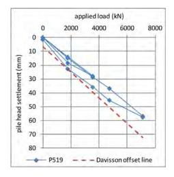
Figure 9. Load versus settlement curve.
