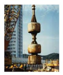
Figure 15. Large diameter RCD drillbit.
