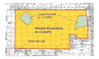
Figure 18. General Excavation near Ground Level.
