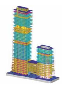
Figure 3: LS-Dyna Analysis Model of the Shenzhen Energy Headquarters Building. © Arup
