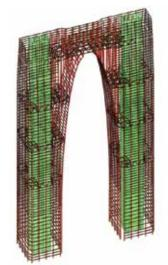
Figure 4: Suzhou "Gate to the East" – structural model for lateral stability analysis. © Arup
