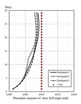
Figure 9. Maximum response of story drift angle (Controlled condition).
