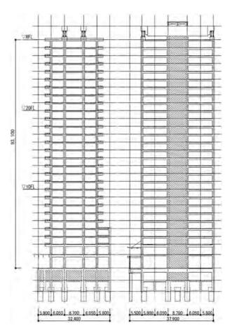
Figure 3. Framing elevation.
