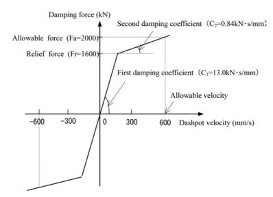
Figure 8. Velocity-force relationship of dashpot.
