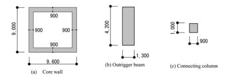
Figure 4. Typical sections of each element.
