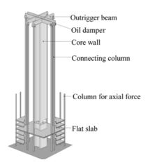
Figure 1. Flexural deformation response control system.
