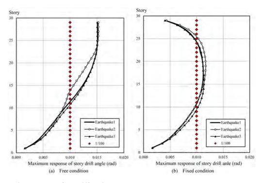
Figure 11. Maximum response of story drift angle.
