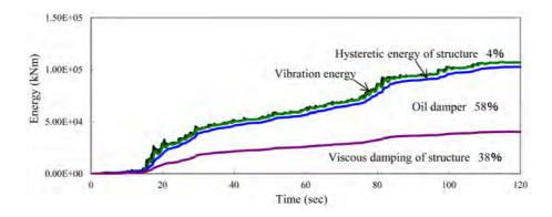
Figure 10. Energy absorption time history (Controlled condition).
