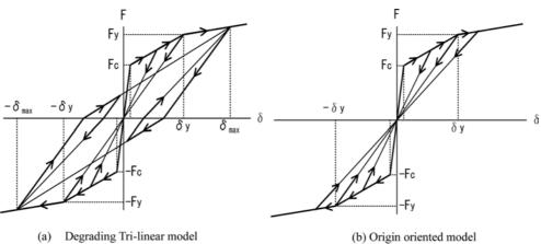
Degrading Tri-linear model
