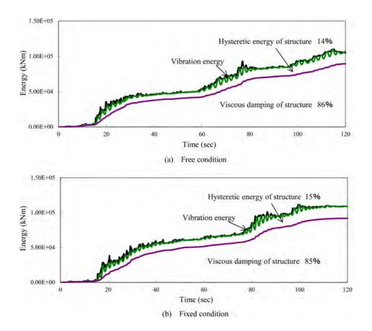
Figure 13. Energy absorption time histories of each element.
