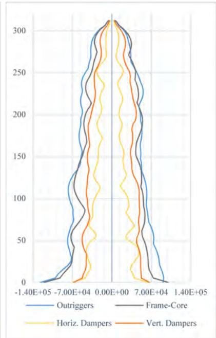
**Figure 13.** Story Shear results for Moderate Earthquake load case.
