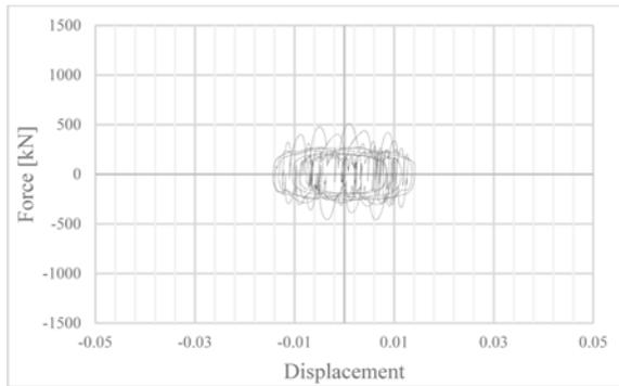
**Figure 16.** Typical force-displacement loop for a damper in the vertical configuration (Moderate Earthquake).
