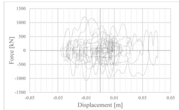
**Figure 17.** Typical force-displacement loop for a damper in the horizontal configuration (Moderate Earthquake).
