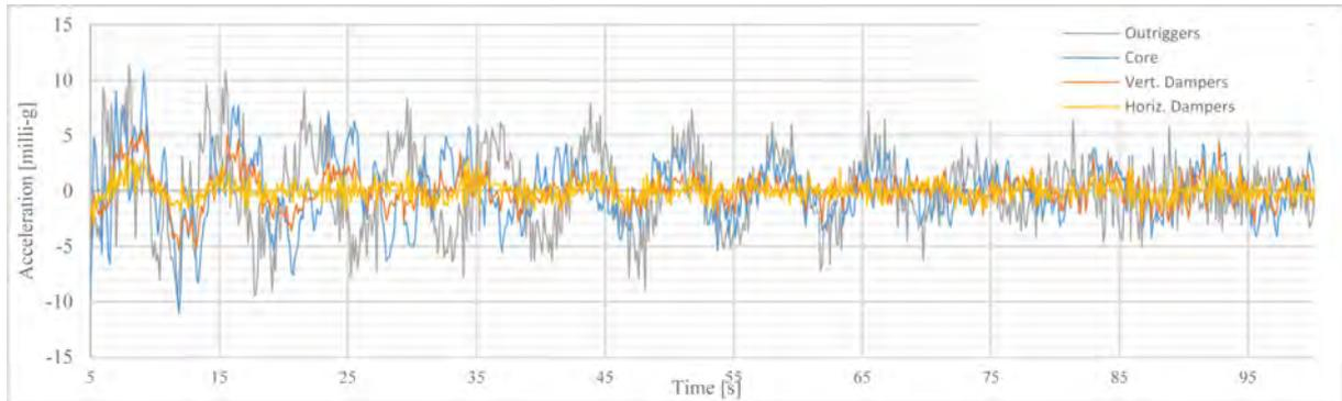
**Figure 14.** Acceleration history at the roof level for the 10-year Wind load case (along-wind direction).
