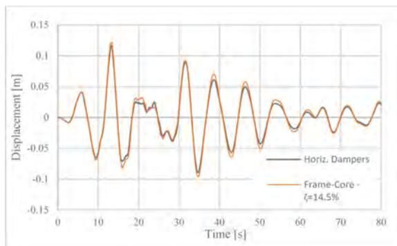
**Figure 18.** Displacement response comparison for computed damping ratio validation (horizontal dampers) - Frequent Earthquake.
