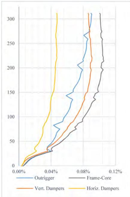
**Figure 11.** Drift results for Frequent Earthquake load case.
