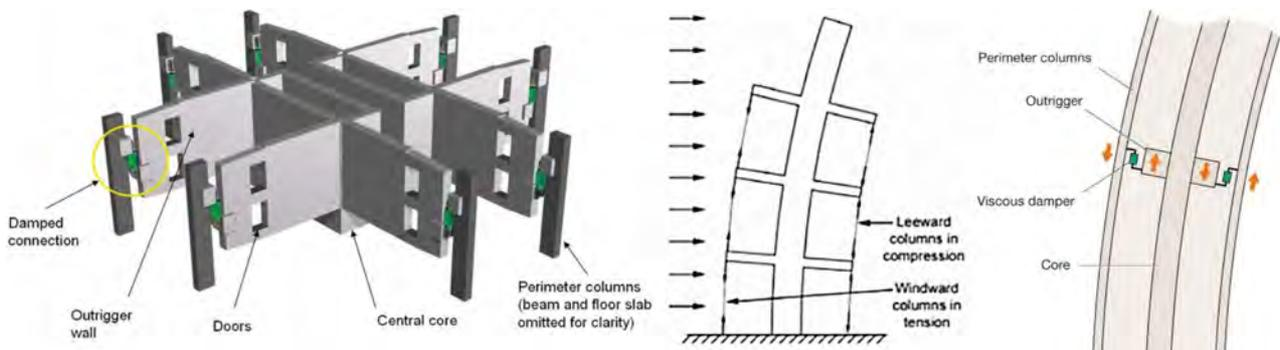
**Figure 1.** The outrigger concept for 60 Story Twin Towers in Manila (Smith and Willford, 2007).
