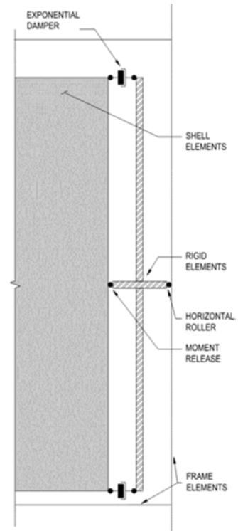
**Figure 10.** Horizontal dampers as modeled in ETABS.
