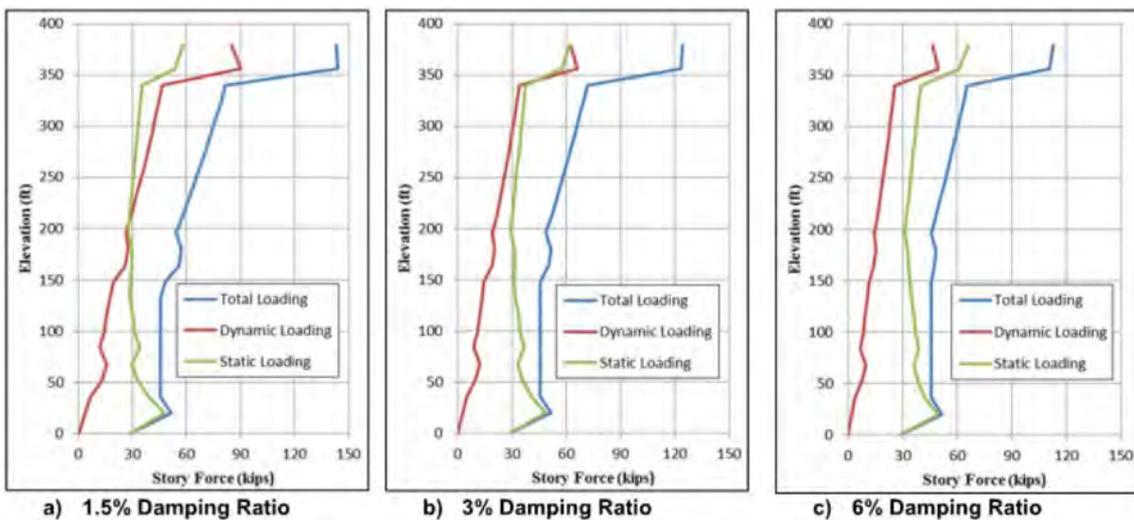
**Figure 4.** Static and dynamic components of wind loads for the San Diego Courthouse project (Sarkisian et al., 2015).
