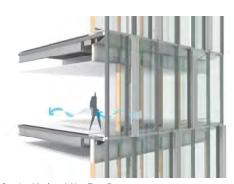
Passive Mode – A Net-Zero Day Heating Flushir Figure 7. The double façade's different modes throughout the year. © Gensler
