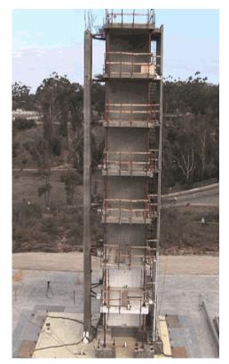
Figure 5. 7-story apartment module on shake table at UCSD's Englekirk Engineering Center (Baumann Research and Development, 2006)
