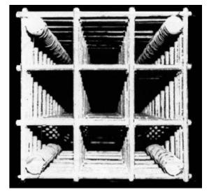
Figure 6. Tests at University of Ottawa showed reduction in rebar and couplers was safe (Baumann Research and Development, 2002
