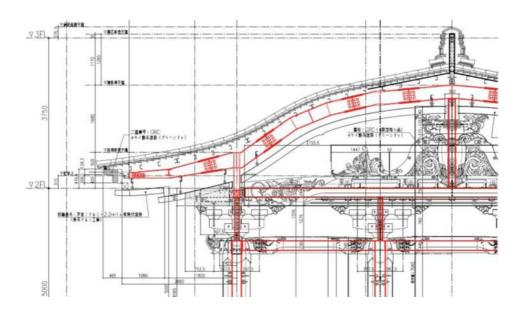
Figure 10. Details of Karahafu-style gable and concealing the structural steelwork.
