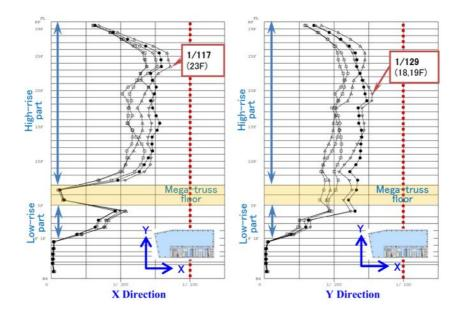
Figure 5. Maximum angle of relative deformation (very rare earthquake level).
