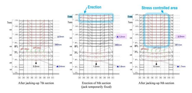
Figure 8. Method of erection above the Mega-truss and displacement control.
