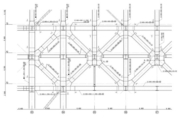
Figure 6. Detail of Mega-truss (Y7).
