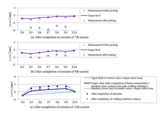
Figure 9. Measurement results before and after jacking.
