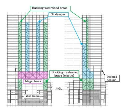
Figure 3. Y7 Elevation.
