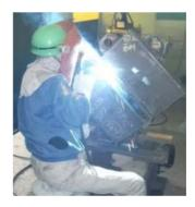
Photo 5. Welding test (inclined vertical).
