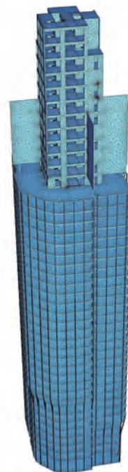
Figure 7. 3-D analytical model of tower (Source: AKT II Limited)
