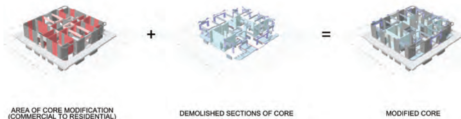
Figure 10. Core modification sequence (Source: AKT II Limited)
