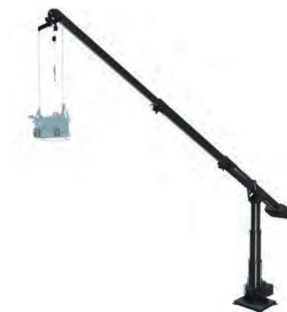
Figure 7. Example: operating BMU BIM model (Source: XS Platforms) 图7. 作业中的BMU BIM模型示例 (来源: XS平台)
