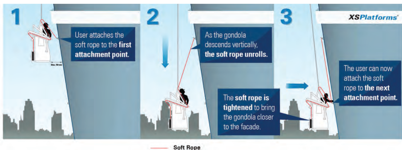
Figure 5. Example: soft rope restraint operation (Source: XS Platforms)
