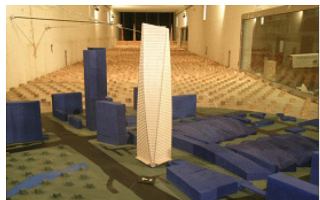
Figure 4. Wind Tunnel Test (source: RWDI)
