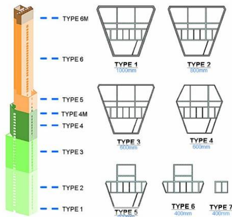
Figure 11. Shape and Thickness of NEATT's Core Wall along the Building Height (source: Arup)
