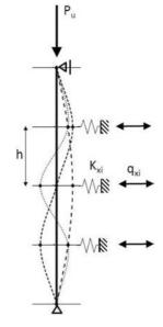
Figure 3. Buckling modes of a multistory column with lateral spring supports.
