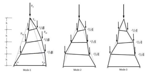
Figure 5. Buckling deformation shape of a single diagrid module.
