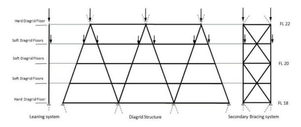
Figure 9. A 2D diagram representing a four story segment of the diagrid structure, leaning structure and secondary bracing system.
