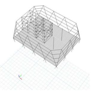
Figure 8. Isometric view of a four story segment of the diagrid structure of Hearst Tower.
