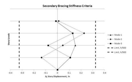
Figure 10. Buckling modes of the diagrid structure.
