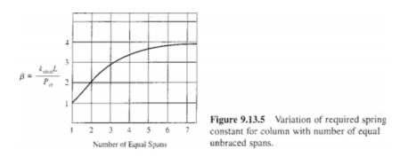
Figure 4. Required spring constant for stability of a multistory column, from Salmon and Johnson, 1980.
