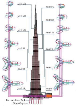
Figure 8. Strain Gage Monitoring System © Samsung C&T
