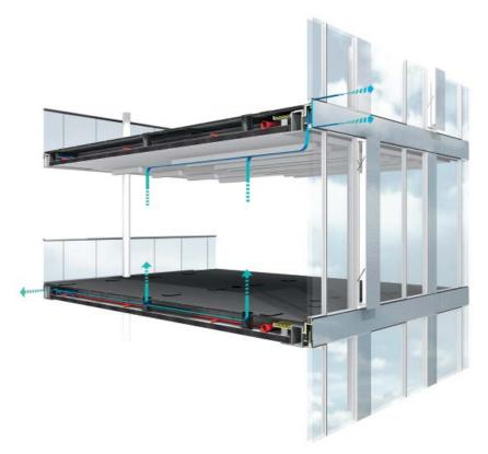
Figure 6. Integrated heating and cooling system inside the new office wings' floor slab
