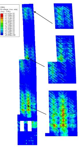
Fig.13 SPSW plastic buckling (tension field action)
