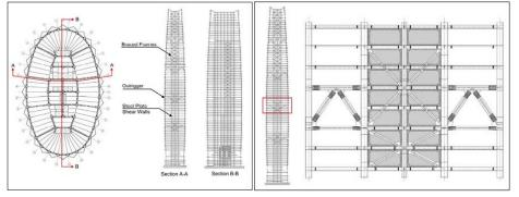
Fig. 2. Typical plan and section
