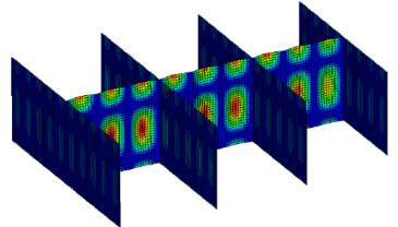
Fig. 10 Introduced imperfections between stiffeners at SPSWs
