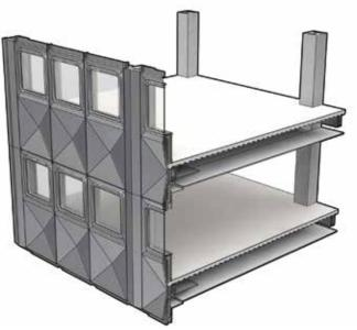
Figure 5. Prudential Building, Chicago (1954) – cladding detail reconstruction.
