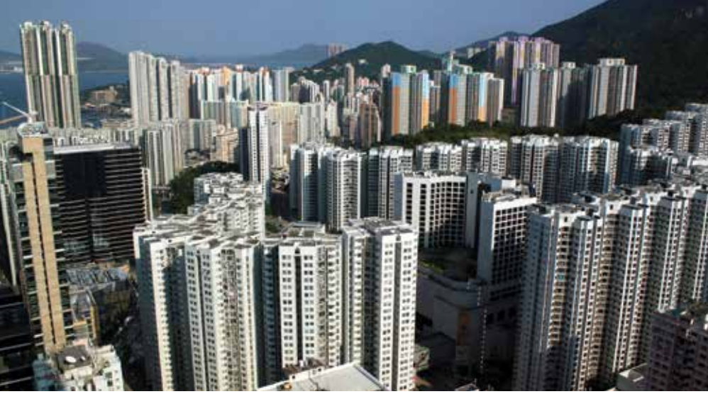
Figure 2. In order to maximize the internal, usable space, developers in Hong Kong could be motivated to simply “extrude” the floor plan, as protruding building features, such as balconies, can count against the total allowable floor area for a building site. © WING (cc by-sa)
