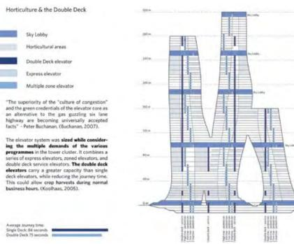
Figure 11. Double Deck Elevator - Tower Diagram
