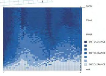
The pixelated matrix (right) is the unfolded skin @ of the tower massing above. Using a combina-tion of environmental softwares a kind of vertical 'land-use mapping' was developed. It shows the light distribution across the threetower skin during a single day. This type of mapping may be utilized to allow the aeroponic modules to become plugged into differing regions of the tower, dependant on seasonality, or crop demand.
